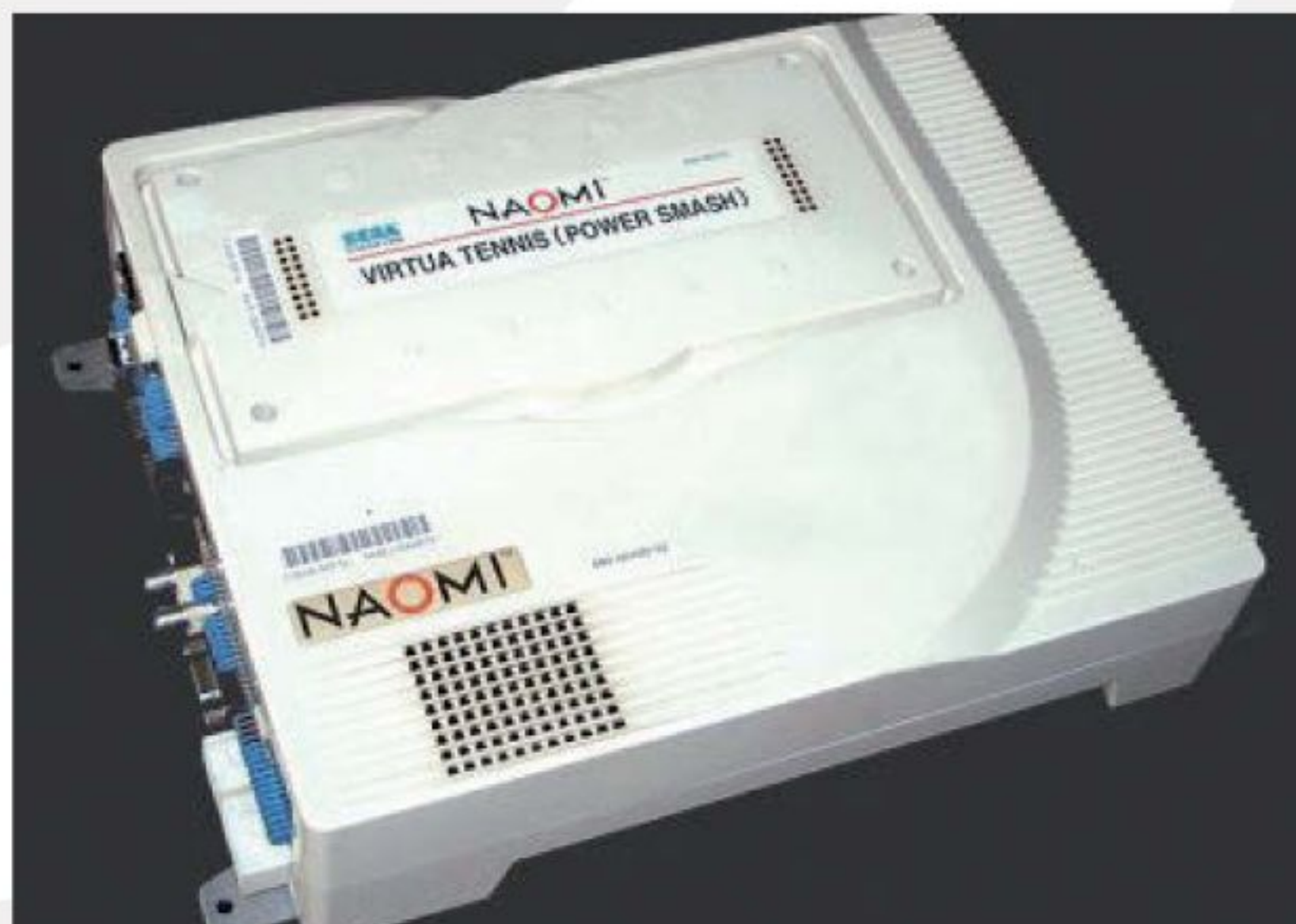
» The NAOMI arcade hardware was essentially a Dreamcast with more memory
