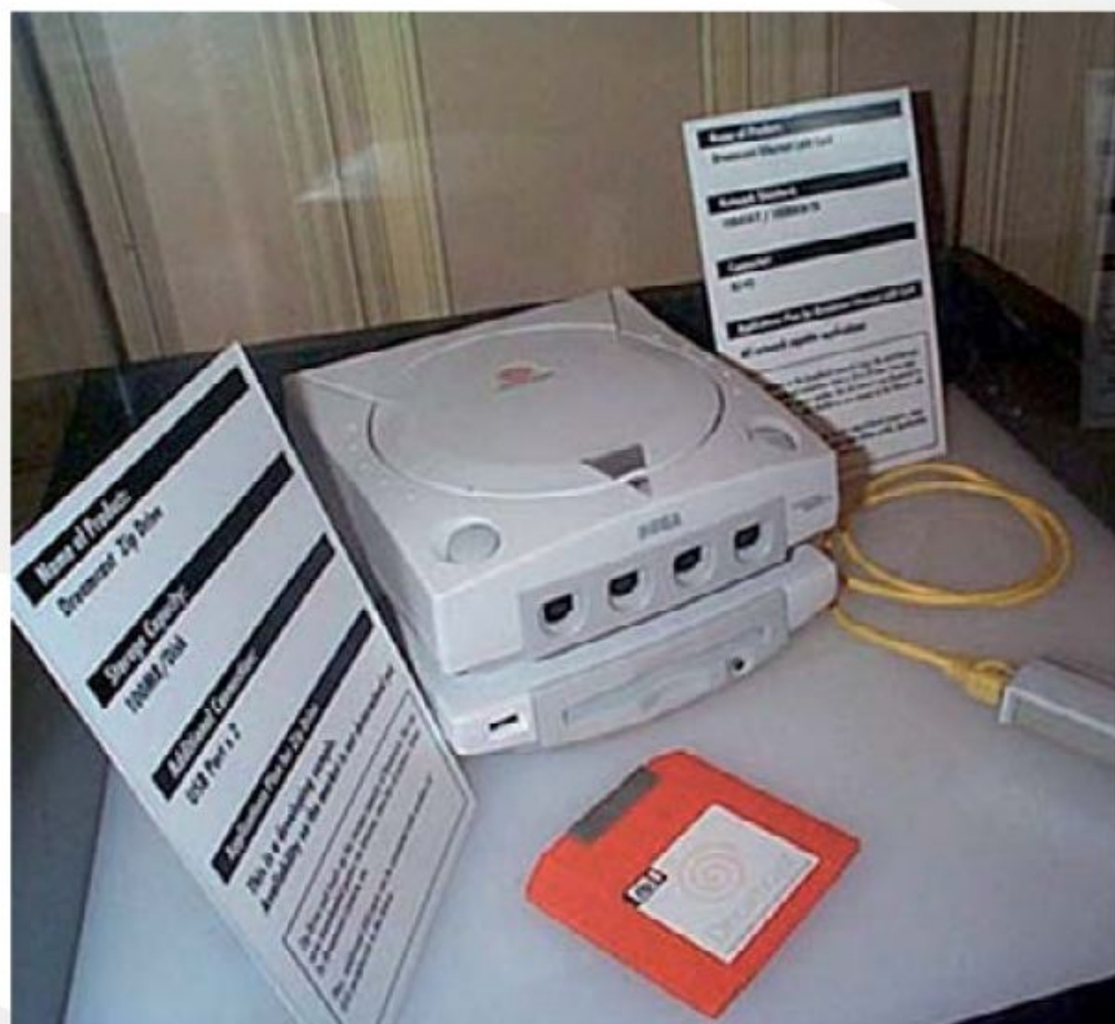
» The proposed Dreamcast Zip drive – sadly it never made it onto the shelves.
