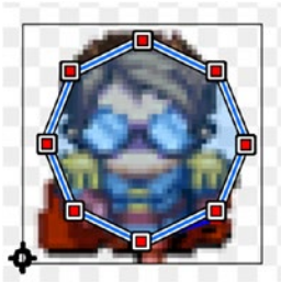
Figure 12-3. The Player sprite's circular collision polygon
