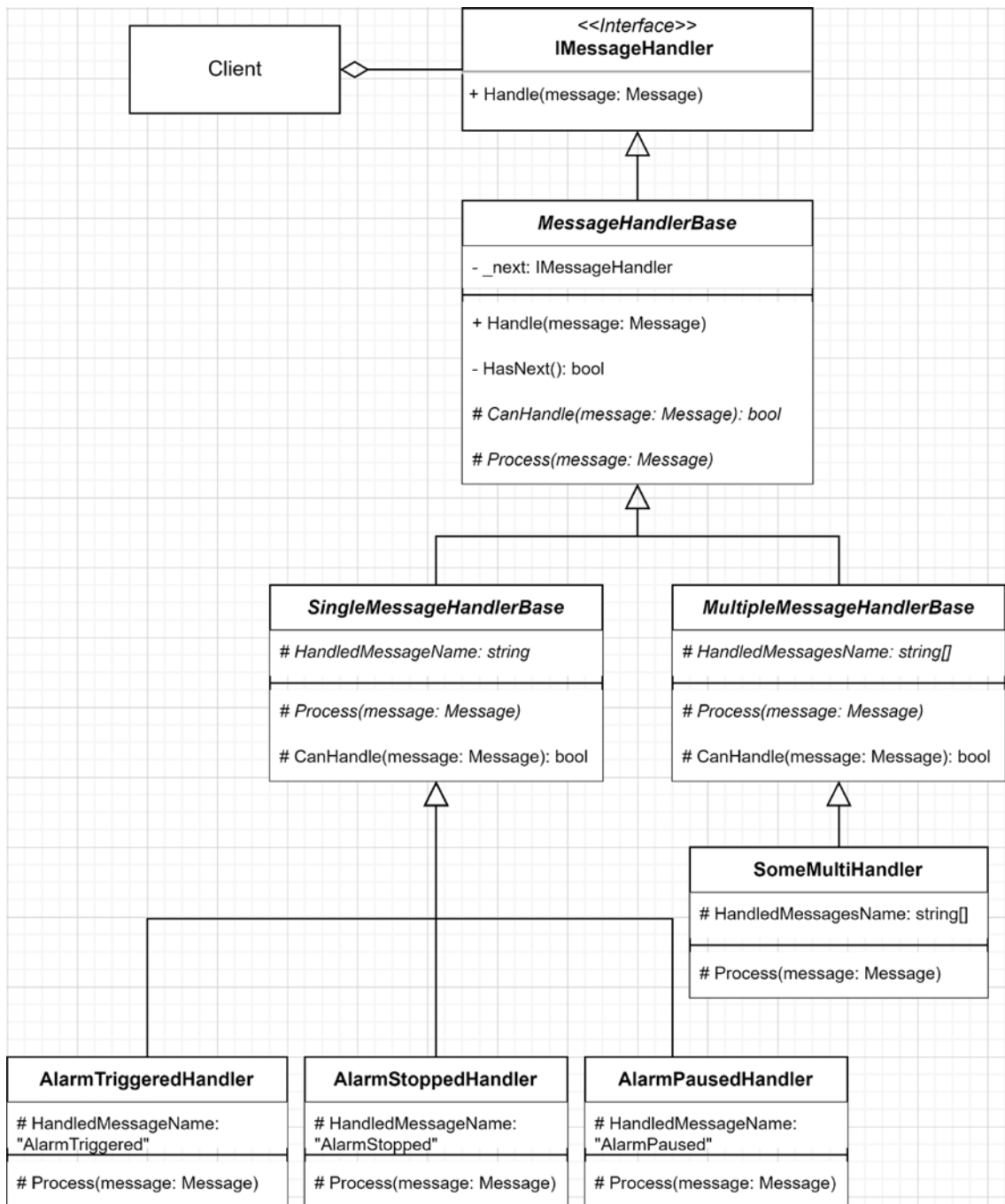
Figure 10.4: Class diagram representing the design of the finer-grained project that implements the Chain of Responsibility and Template Method patterns
