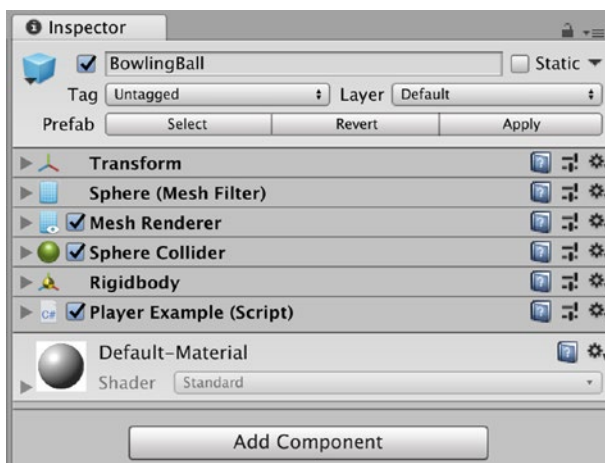
Figure 8-4. The properties of the BowlingBall prefab
